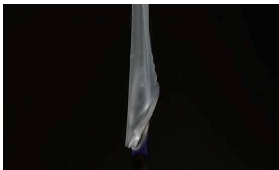
6% loading to PP (100 \mu m VTM-0)
